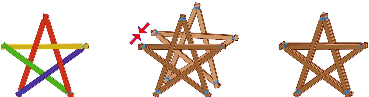
Notice that the center of the star frame is a pentagon. With the stars securely tied together with rubber bands, pull apart the center of the frame. Place one peg at each of the point of the pentagon. To secure the pegs we need to use hot glue. Put the hot glue where the peg meets the frame. Be sure to get both sides of the peg. Now we have a completed Parol frame.
